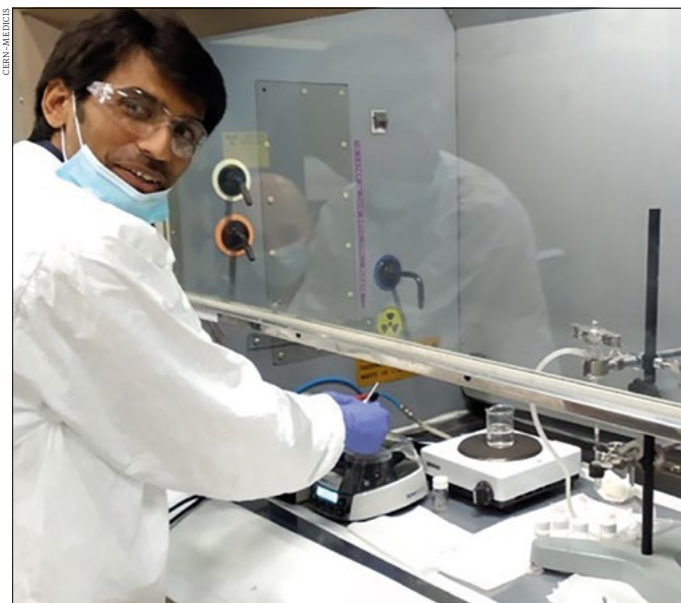
Purified Radiochemistry set-up (above) for the separation of low-activity radioisotopes at CERN's MEDICIS facility.
