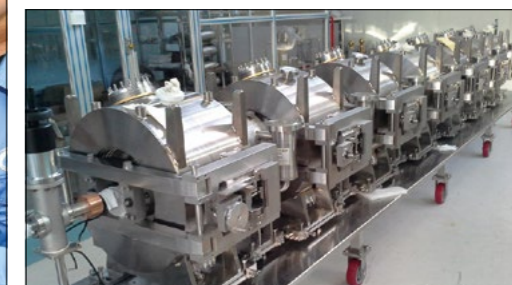
Big science, lasting legacy Over the past 20 years, IHEP's accelerator division has overseen a number of large-scale accelerator initiatives in China. Left: RFQ commissioning at the China Spallation Neutron Source (CSNS). Top: two CW proton superconducting cavity modules (comprising seven cavities per module – shown below) for the Accelerator Driven Sub-critical System (ADS).
